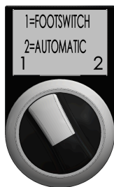
Figure 24: Automatic lid switch
